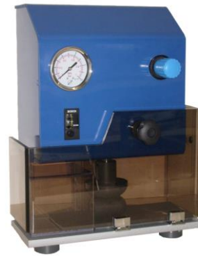
ACRN – ATS Tube Seal Tester
