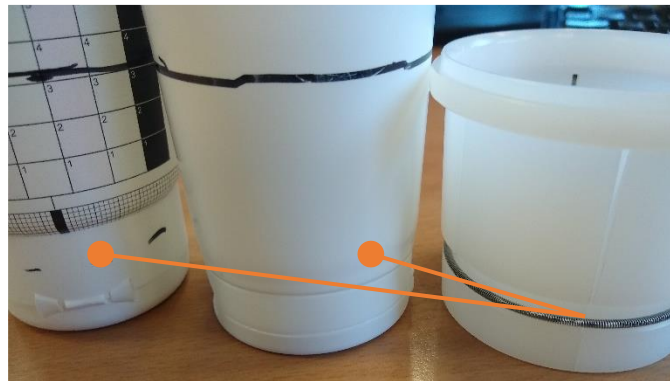
(LEFT) Fit over cap, on standard tube (CEN) Fit over tube body, in tube with low-profile cap
